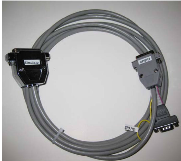
Figure A1 – GPS-RT to GPSSIM-14 Interface Cable
